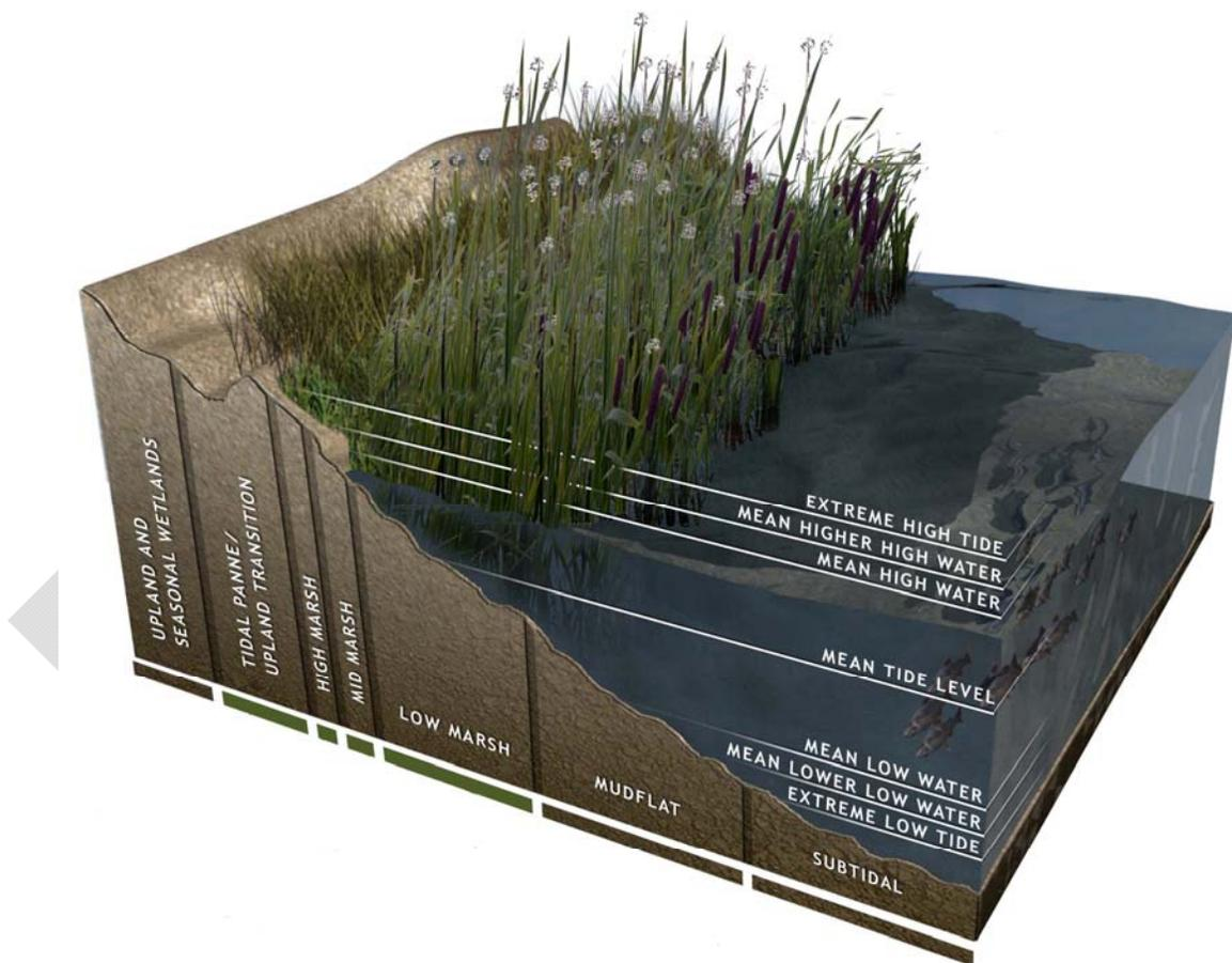
**Figure 2. Typical cross section through a marsh.**
