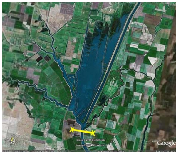
Figure 5. Effect of Liberty Island Levee Breach on Channel Geometry at Cache Slough
