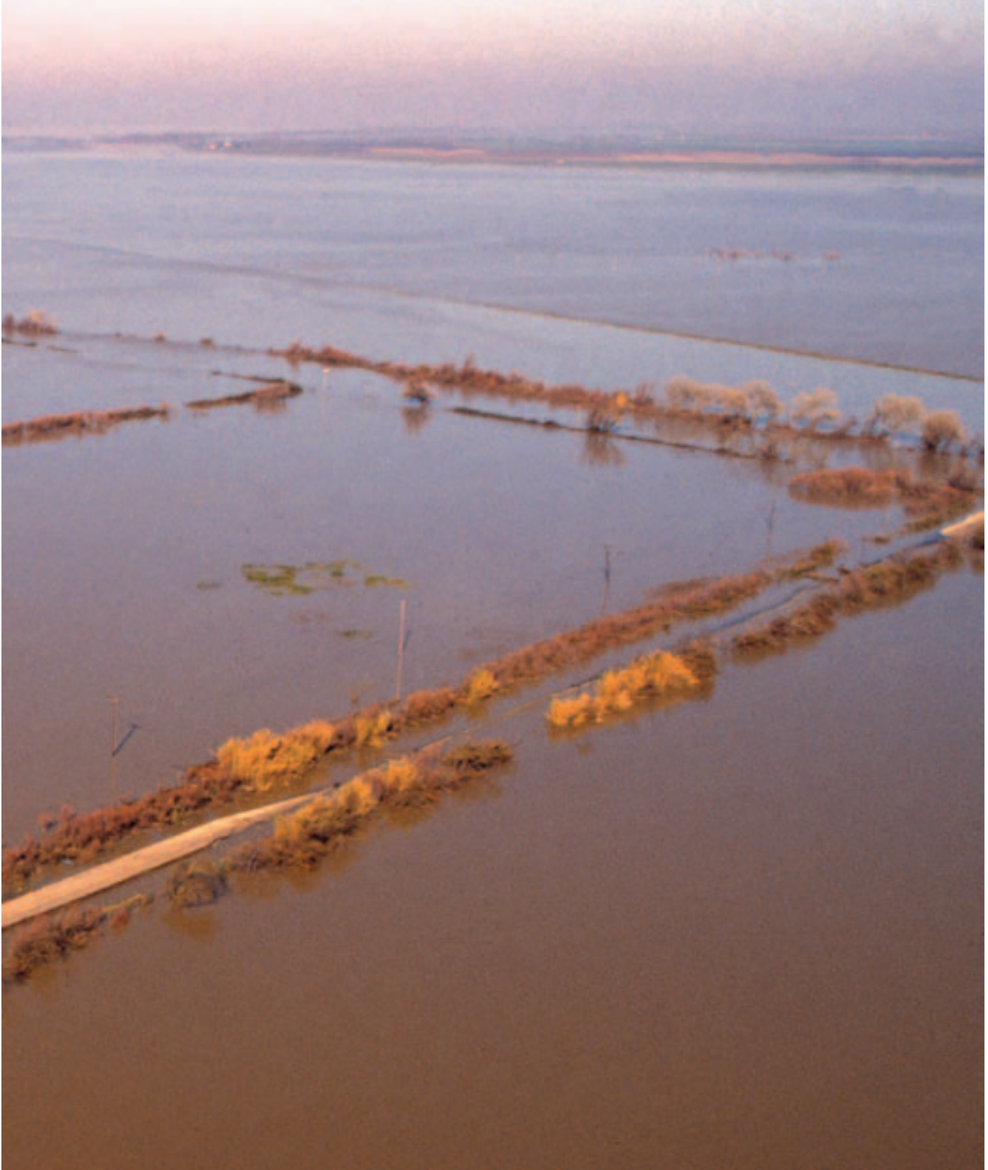
The Yolo Bypass is an example of successful multi-objective floodplain management. Established as a floodwater corridor, it is also intensively cultivated and parts of the bypass provide outdoor recreation and spawning and rearing areas for native fish. (DWR photo)
