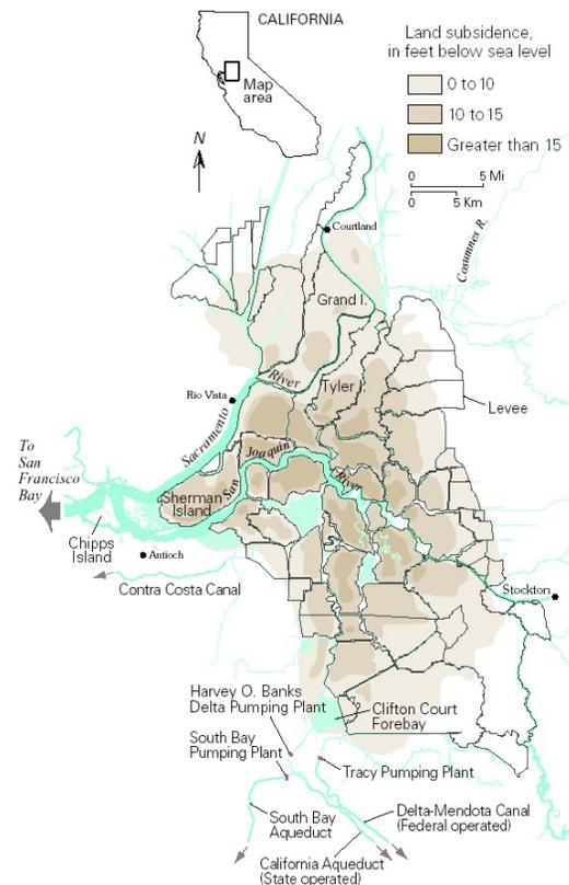
**FIGURE 1 – Sacramento-San Joaquin Delta, California.** The Delta is comprised of islands or tracts protected by an extensive levee system. Shading indicates the elevation of subsided islands. (Adapted from Ingebritson et al. 2000).
