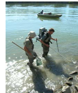
Darell Slotton and Shaun Ayers, UC Davis, electro-shock small fish for mercury sampling to examine mercury patterns in the food web.
